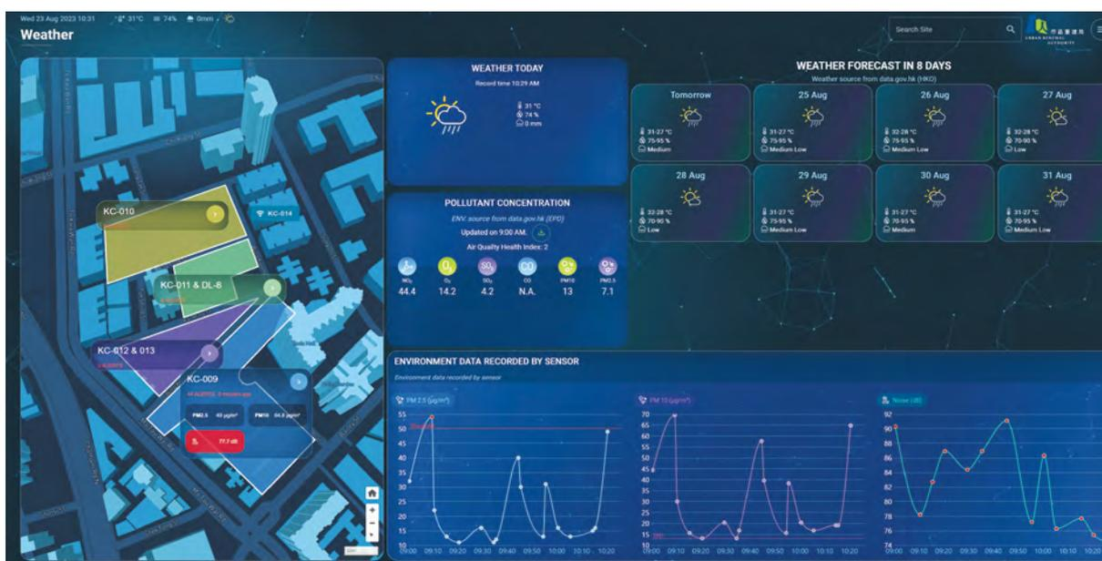
The Environmental Monitoring Module of the DCMP collects real time environmental data including noise and pollutant levels from different construction sites for URA staff's monitoring from their offices.
